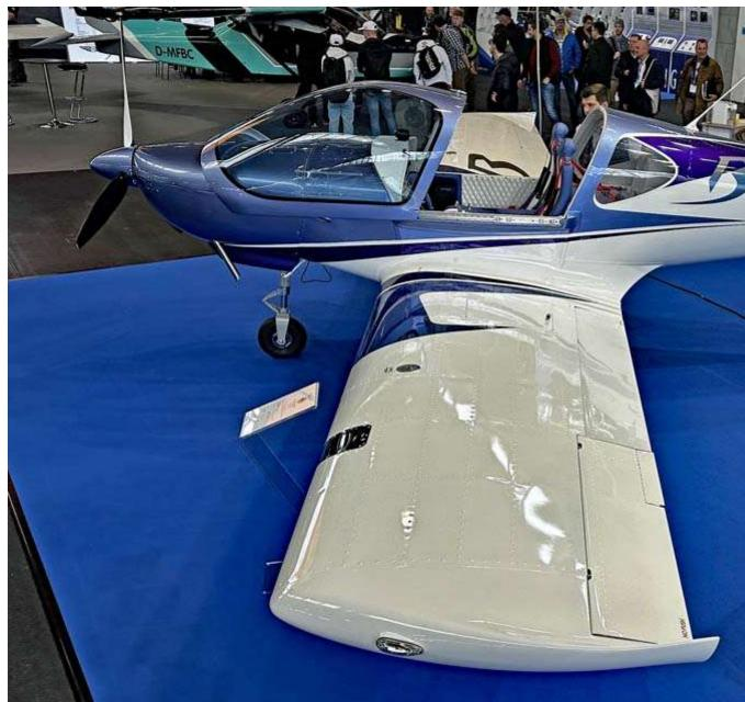
[Dan Johnson]"DW200 is a two-seat, all-metal, low-wing aircraft with sideby-side seats," said Belmont. "The landing gear consists of a fixed tricycle landing gear with steerable nose wheel."
