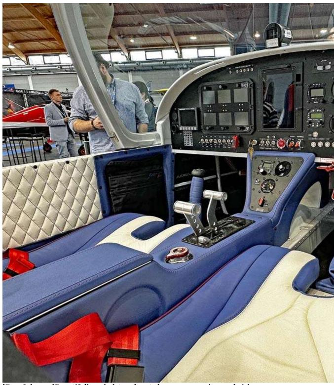
[Dan Johnson]Beautifully upholstered seats have a composite sandwich structure. Four-point seat belts are standard. Headphone jacks are located behind the pilot's seats.
